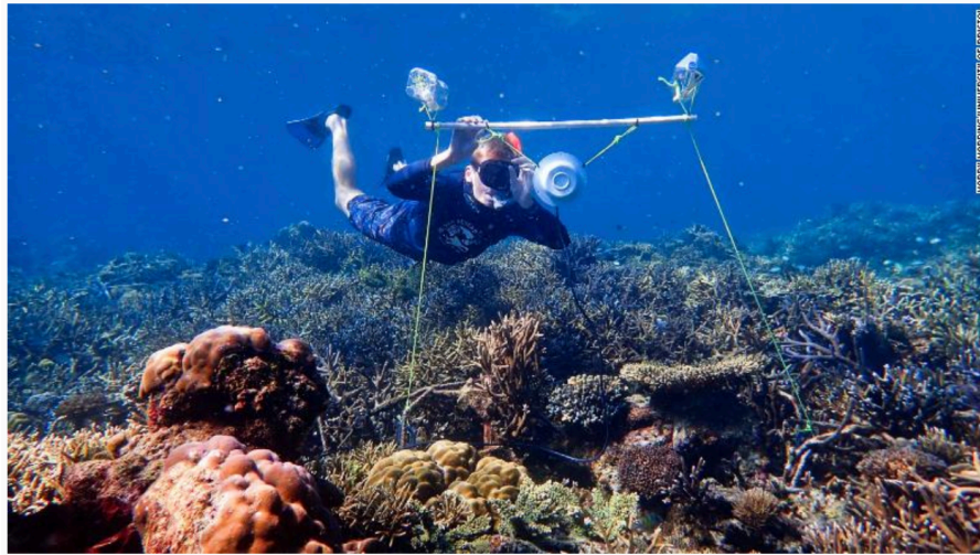
Researcher Tim Gordon deploys an underwater loudspeaker on a coral reef.
